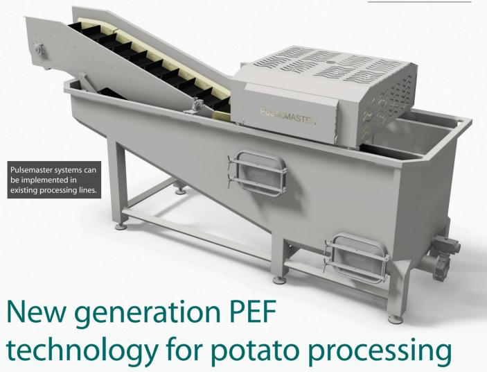
The innovative Dutch company Pulsemaster recently introduced a new generation PEF (pulsed electric field) technology claiming that it can significantly improve potato processing. The Pulsemaster PEF technology induces poration of potato cells, leading to cell disintegration. This makes the pulsed electric field systems an alternative to preheaters in the potato industry.
